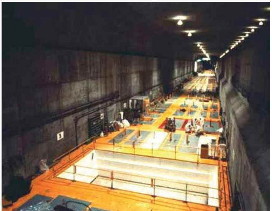
The canyon deck of the 820-foot-long 221-B plutonium processing plant at Hanford, which produced weapons plutonium during World War II.
