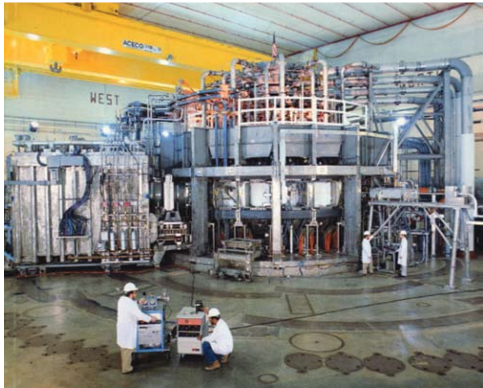
Princeton’s Tokamak Fusion Test Reactor (TFTR) was conceived as a link between its generation of tokamaks and the first experimental power reactor. It reached record plasma temperatures of 200 million degrees in July 1986 with deuterium fuel, and two years later reached 510 million degrees using deuterium-tritium fuel. But budget cuts precluded further breakthroughs, and the TFTR was decommissioned early, in 1995.
