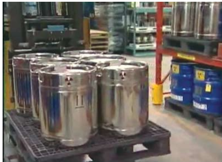
A moly “cow,” which is milked to supply the short-lived isotope technetium-99m for medical diagnostic procedures.
