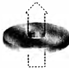
(g) Flat, washer-shaped magnetic toroid begins to simulate the ideal Ampèrian current element of (c)
