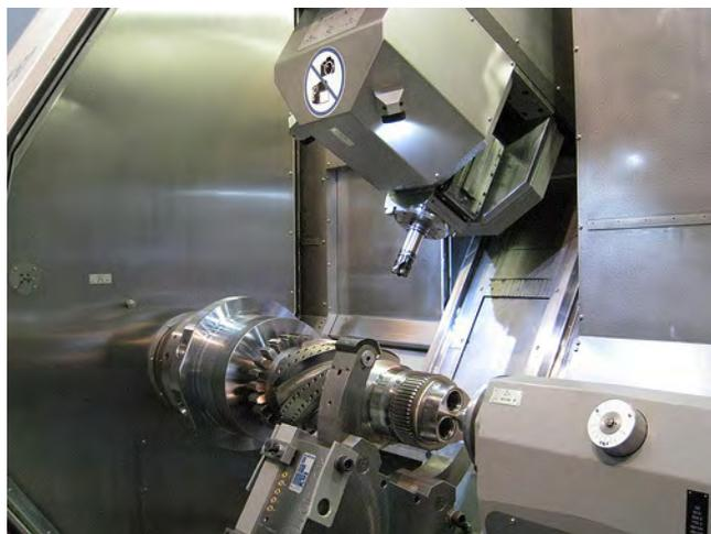
*A CNC machine tool. Such automated devices can automatically change cutting tools and reposition work objects, allowing for high automation of part-machining.*
