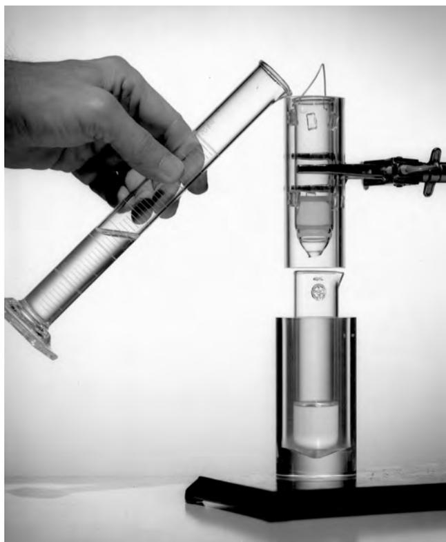
*The first chemical separation of technetium-99m from molybdenum-99.*
