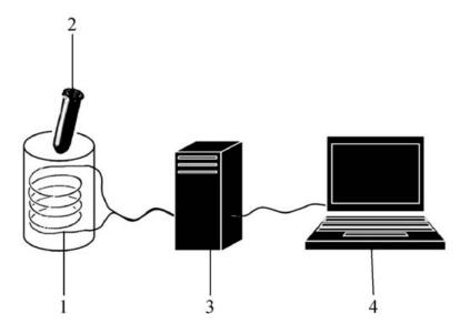
**Fig. 1** Device for the capture and analysis of electromagnetic signals (EMS): (1) Coil: a bobbin of copper wire, impedance 300 Ohms; (2) Plastic stoppered tube containing 1 mL of the solution to be analyzed; (3) Amplifier; (4) Computer with software.
