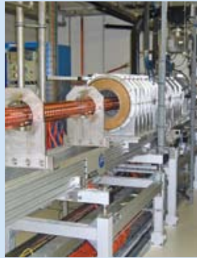
The linear accelerator (linac) at the Australian Synchrotron in Clayton, Victoria.
