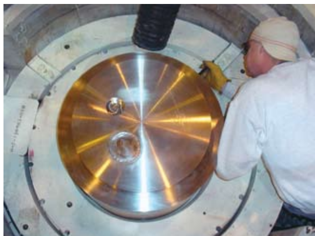
The first Shippingport Spent Fuel Canister (SSFC) being welded for storage in underground vaults at the Canister Storage Building, where they will stay until permanent burial—instead of being used to produce radioisotopes.
