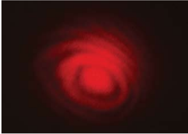
The interference pattern produced with a Michelson interferometer using a red laser.
