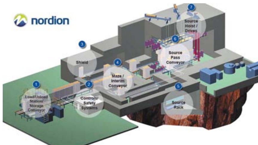
An interactive illustration of a gamma ray irradiator (using cobalt as a source). The product moves on a conveyor belt past the irradiation source, where it receives a pre-programmed and timed exposure.
