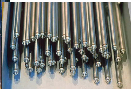
A nuclear fuel assembly (left). The long tubes are zirconium-alloy-clad fuel rods which are fastened together into large bundles that form the core of a nuclear reactor. Uranium oxide fuel pellets are stacked inside each rod. Individual fuel rods are shown in the inset.
