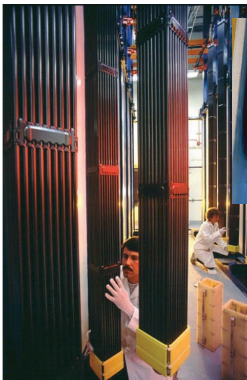
A nuclear fuel assembly (left). The long tubes are zirconium-alloy-clad fuel rods which are fastened together into large bundles that form the core of a nuclear reactor. Uranium oxide fuel pellets are stacked inside each rod. Individual fuel rods are shown in the inset.
