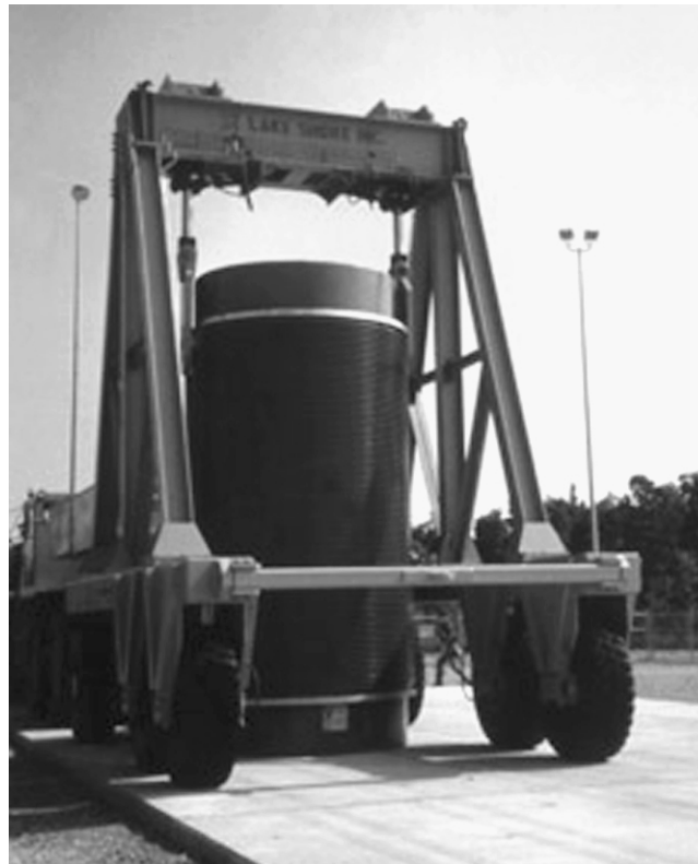
A dry storage cask for spent fuel at the Surry Nuclear Power Station in Virginia. Each dry cask is 16 feet high, 8 feet in diameter, and has 15-inch-thick walls made of steel. Each cask holds 21 to 24 spent fuel assemblies.
