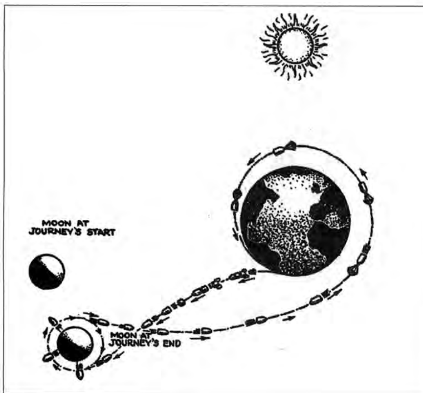
This 1930 drawing of the trajectory astronauts would take from the Earth to the Moon is very familiar, in that it is the figure "8" employed nearly 40 years later in the Apollo program.
