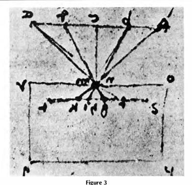
**LEONARDO'S DIAGRAM OF THE PRINCIPLE OF THE CAMERA OBSCURA** The object is abcd (written backwards, on the top line). From it, rays go through the small hole mn, cross, and then diverge onto a sheet of paper, st. The image is reversed from right to left, and is upside down.
