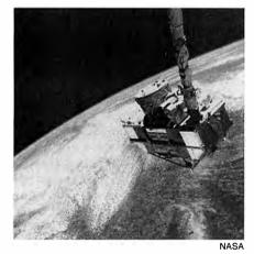
Crista-Spas, the Cryogenic Infrared Spectrometers and Telescopes for the Atmosphere (Crista), housed on the Shuttle Pallet Satellite (Spas), is shown here in a check-out phase on the robotic arm of the Space Shuttle.
