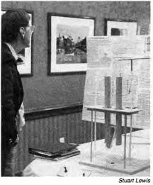
Students today must relive the process of discovery of new physical principles made by past discoverers, and learn the method for making valid new discoveries of principle, as LaRouche discusses (p. 46). Here, a model of Ampère's Second Equilibrium Experiment, constructed by Bob Bowen for the Schiller Institute.
