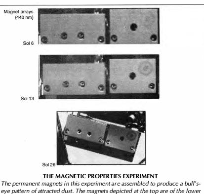
eye pattern of attracted dust. The magnets depicted at the top are of the lower magnet array on the Pathfinder lander on Sol 6, its sixth day on Mars. The strongest magnet, on the right, shows slight evidence of dust collected. The middle photograph, on Sol 13, shows a more pronounced pattern. The lower set of magnets are mounted higher up on the lander, and on Sol 26, show that more dust has been attracted to the magnet.
