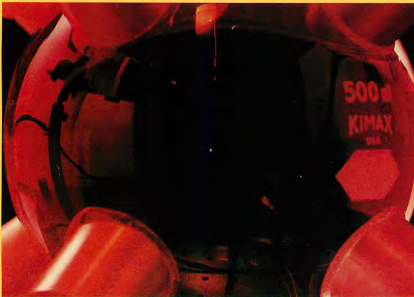
Time-lapse photograph of a sonoluminescence experiment at Lawrence Livermore National Laboratory. Transducers surround a 500-milliliter flask with a flash of light in the center.
