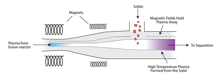
Schematic of Fusion Torch Processing of Solid Waste
