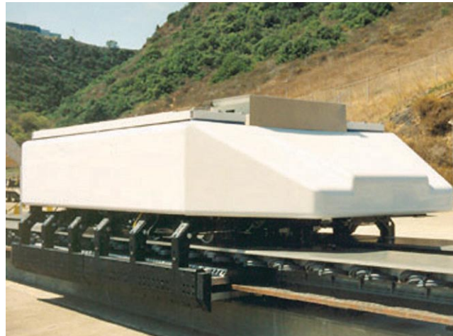
The General Atomics full-scale Inductrack test vehicle on the first section of its test track.
