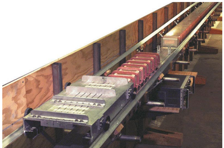
The 20-meter, scale-model test track used to test the Inductrack concept at LLNL. The test cart and electric drive circuit are in the foreground.
