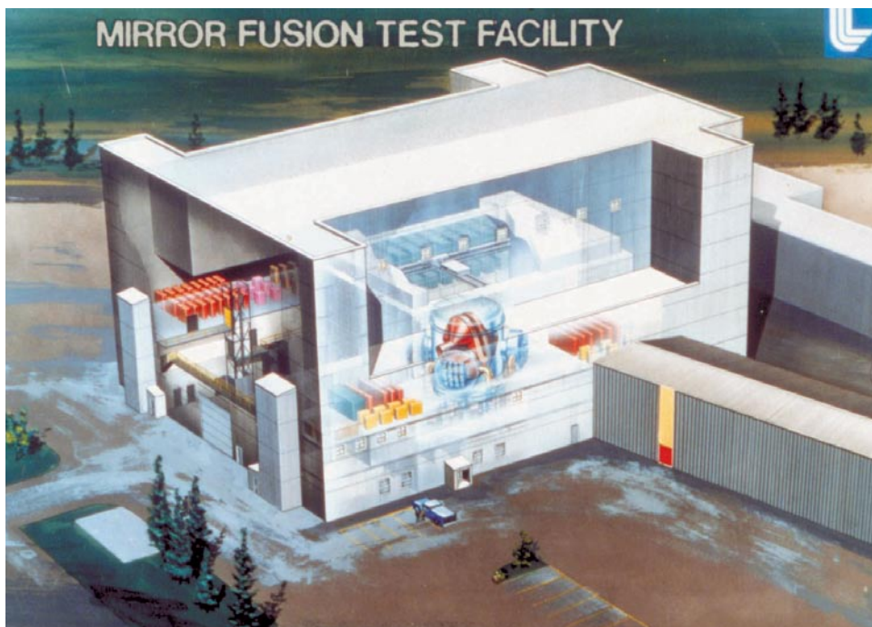
Artist's drawing of the Mirror Fusion Test Facility (MFTF), built at Lawrence Livermore National Laboratory in the 1980s. The vacuum vessel at center is shielded in a seven-story-high concrete vault. The MFTF was forced to shut down soon after it was fully completed because of budget cuts. The U.S. magnetic fusion program was then narrowed to concentrate on tokamaks.
