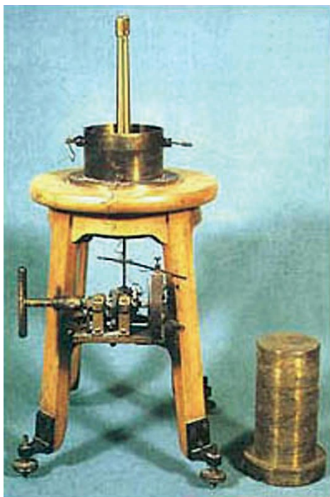
The Curie electrometer, invented by Pierre Curie and his brother, Jacques, used a quartz electrobalance to detect extremely small changes in electrical currents produced when rays from uranium ionize the surrounding air.
